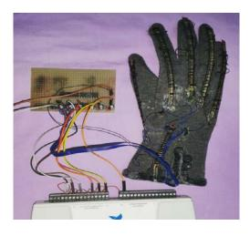
Figure 9: sensory glove hardware circuit
