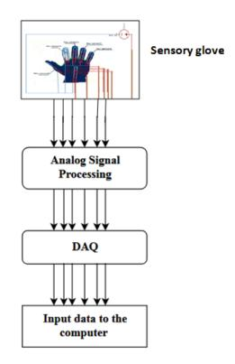
Figure 10: block diagram of the sensory glove system
