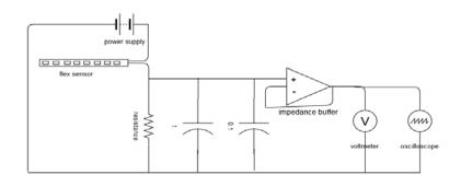
Figure 12: the second electrical circuit for flex sensor
