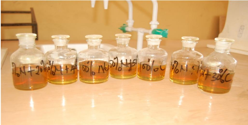
**Plate 3:** Formulated cutting fluids
