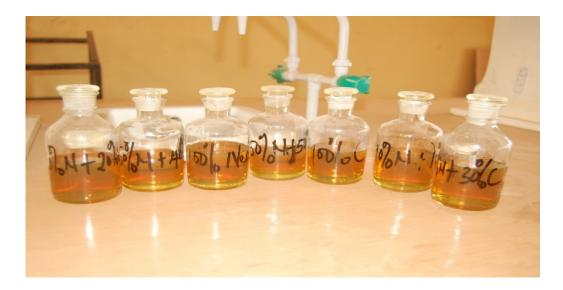
Plate 3: Formulated cutting fluids
