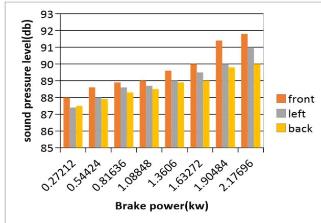
Figure 6: sound pressure level of B25+LPG at different locations
