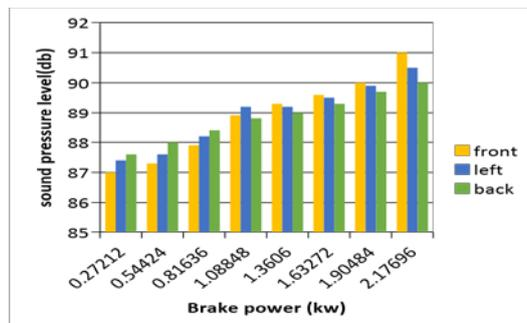
**Figure 5:** Sound pressure level of B25 at different locations
