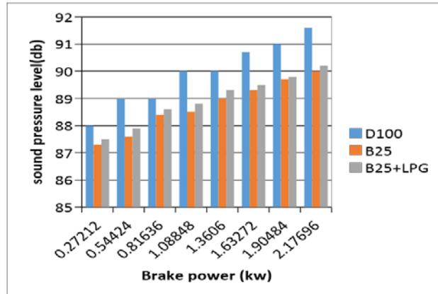
**Figure 9:** Comparative results of sound pressure level at back positions
