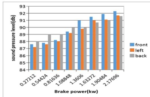
**Figure 4:** Sound pressure level of D100 at different locations
