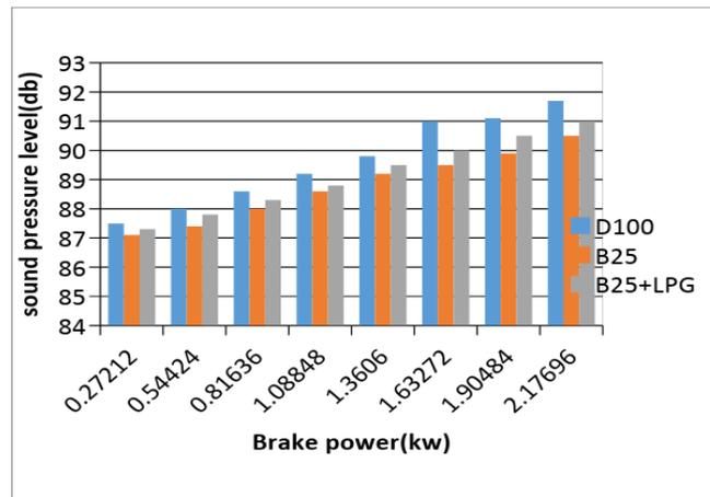
Figure 8: Comparative results sound pressure level left position
