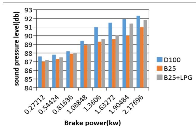
Figure 7: Comparative results of sound pressure level at front positions
