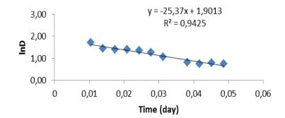
Figure 11: Determination of K<sub>2</sub> by carrying lnD as a function of time (days)
