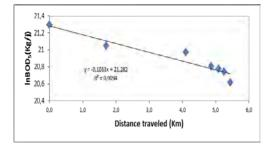
Figure 10: Determination of J1 by carrying ln BOD5 (kg / d) as a function of distance traveled
