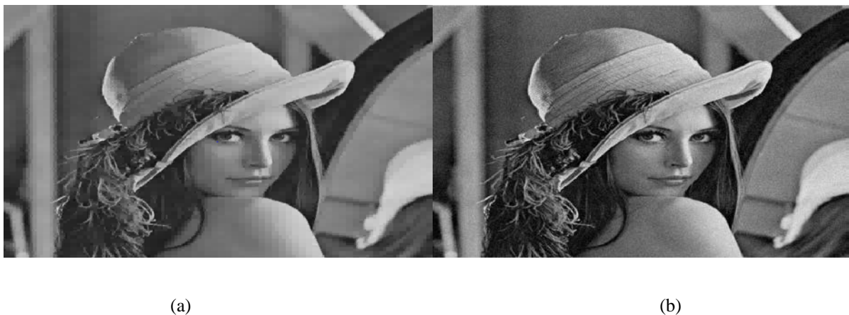
Figure 5: (a) Noisy Lena image with low-level Gaussian noise; variance = 0.001 & mean = 0, (b) The corresponding reconstructed Lena image using conventional wavelet de-noising by thresholding; Correlation = 0.98 and PSNR = 29.51 dB.
