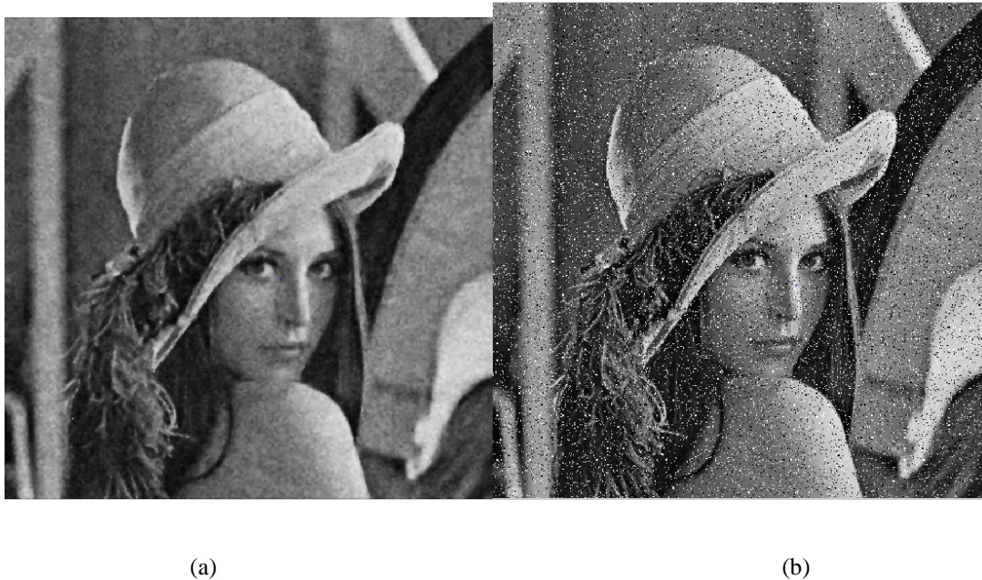
Figure 13: (a) Noisy Lena image with a high-level noise density of 0.1 (salt and pepper noise), (b) The corresponding reconstructed Lena image using circular wavelet de-noising scheme; Correlation = 0.9733 and PSNR = 26.4267 dB.
