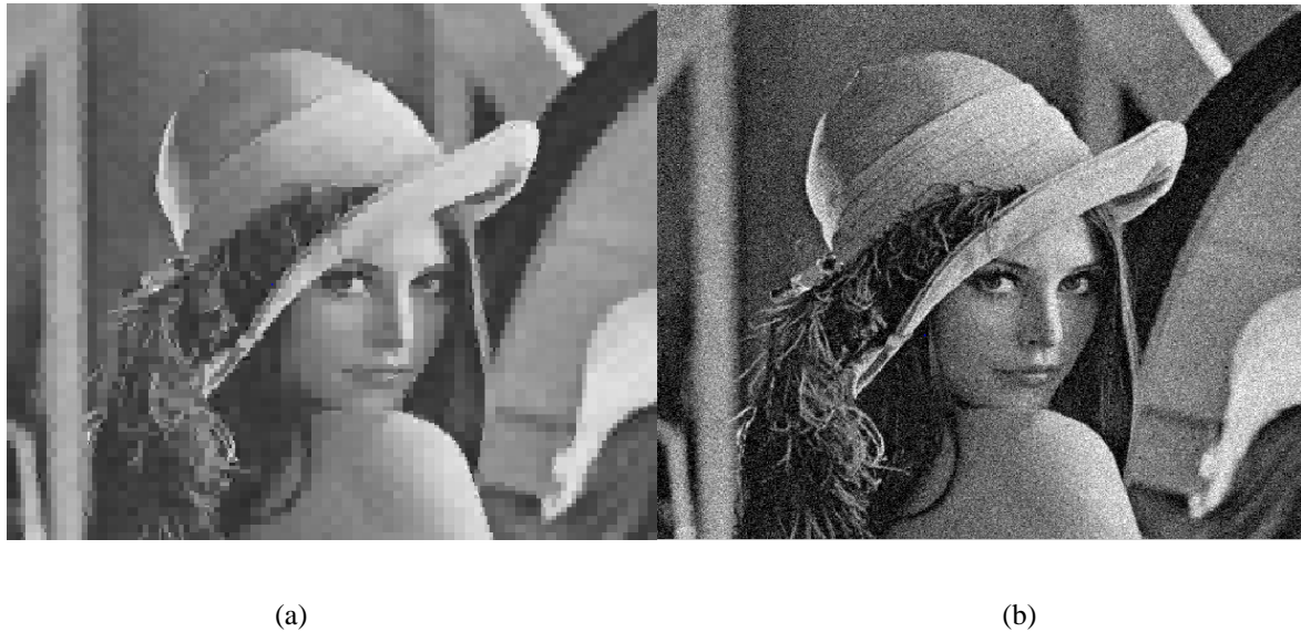
Figure 6: (a) Noisy Lena image with mid-level Gaussian noise; variance = 0.01 & mean = 0, (b) The corresponding reconstructed Lena image using conventional wavelet de-noising by thresholding; Correlation = 0.96 and PSNR = 25.12 dB.
