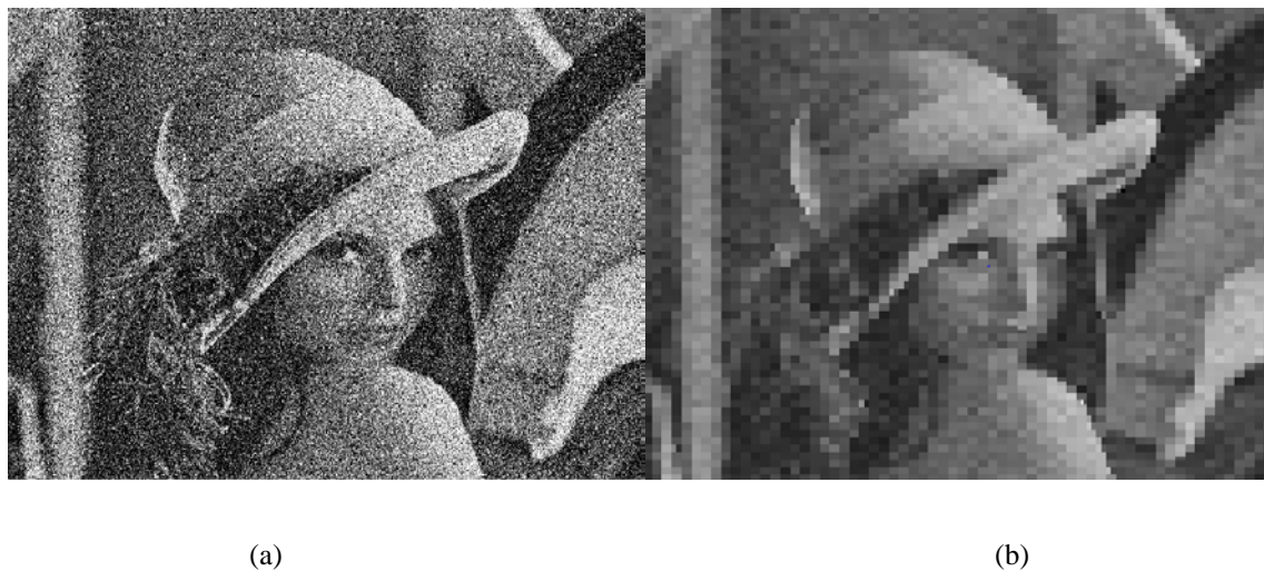
Figure 7: (a) Noisy Lena image with high-level Gaussian noise; variance = 0.1 & mean = 0, (b) The corresponding reconstructed Lena image using conventional wavelet de-noising by thresholding; Correlation = 0.91 and PSNR = 21.04 dB.
