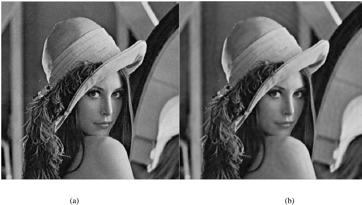
Figure 8: (a) Noisy Lena image with low-level Gaussian noise; variance = 0.001 & mean = 0, (b) The corresponding reconstructed Lena image using circular wavelet de-noising scheme; Correlation = 0.9921 and PSNR = 31.6530 dB.
