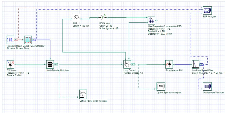
**Figure 7:** Simulation system of the calculation of dispersion in fiber optics
