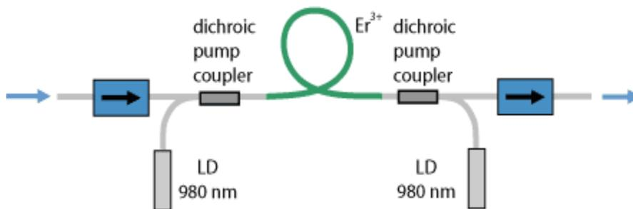
**Figure 6:** Schematic setup of a simple erbium-doped fiber amplifier.
