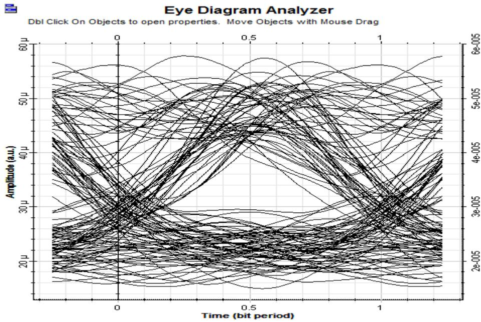
Figure 10: Eye diagram at 180km fiber length equal to  $0.17 \times 10^{-5}$
