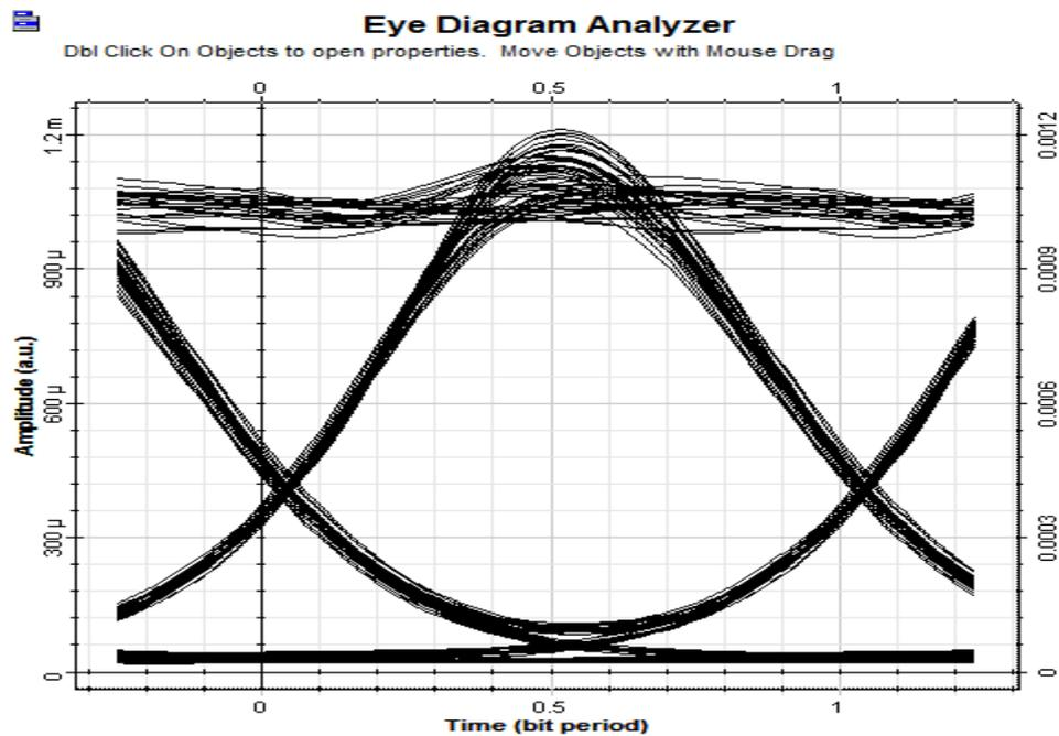
Figure 11: Eye diagram at 50 km fiber length equal to  $5.29 \times 10^{-52}$
