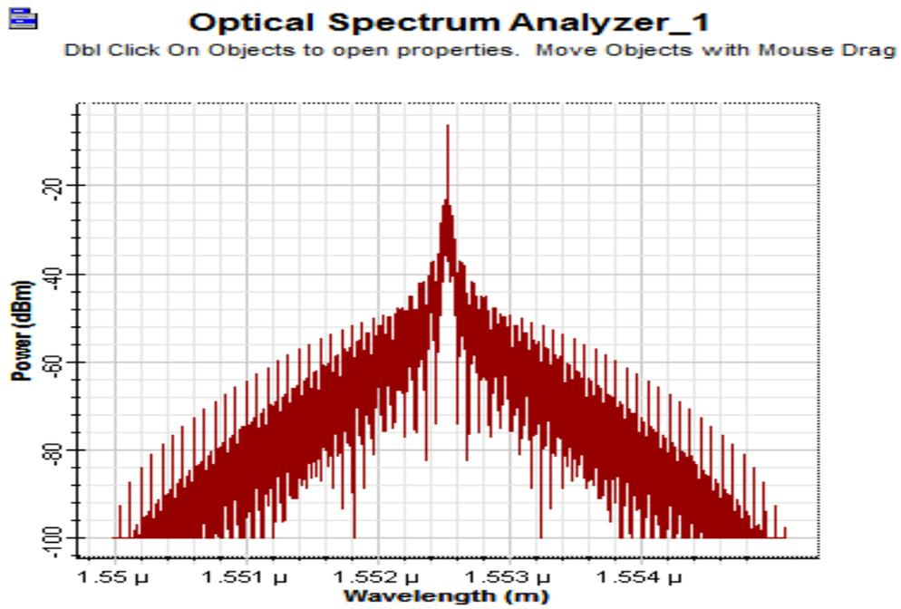
Figure 12: Optical spectrum at the transmitter channel
