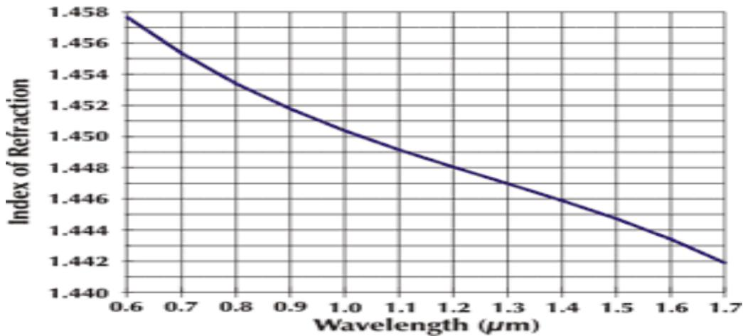
**Figure 3:** Refractive Index of Fused Silica
