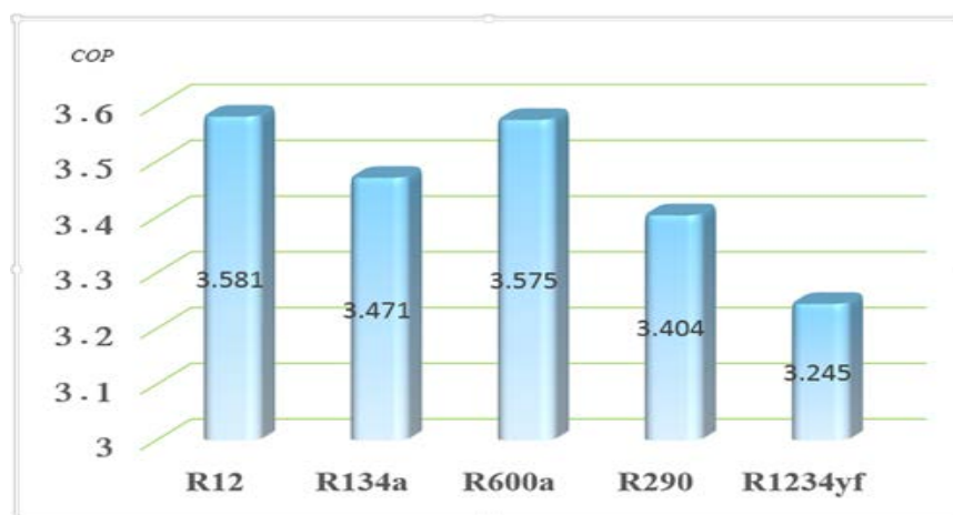
Figure 3: Shows the COP of R12 and R134a comparison with alternative refrigerants.
