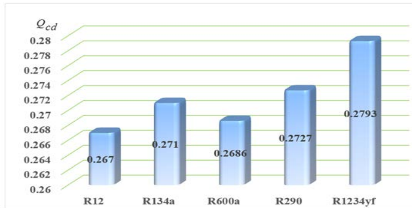
Figure8: Shows the Q_{cd} of R12 and R134a comparison with alternative refrigerants
