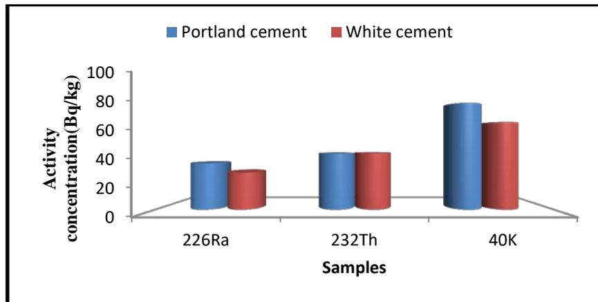
**Figure 1:** Comparison between the average activities of <sup>226</sup>Ra, <sup>232</sup>Th and <sup>40</sup>K of Portland and white cement samples under investigation.
