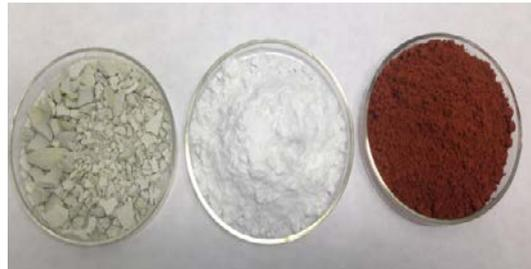
**Figure 3:** rare earth hydroxide, rare earth oxalate and rare earth oxide
