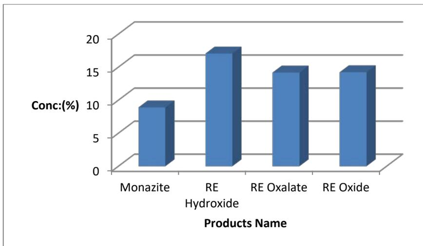
**Figure 8:** Various concentration of  $\text{Nd}_2\text{O}_3$  in rare earth oxide processing
