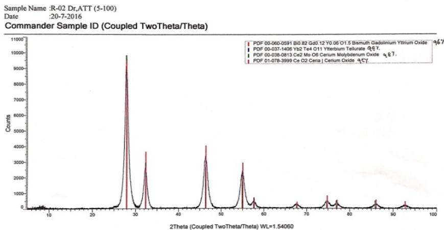
**Figure 5:** XRD chart of rare earth oxide
