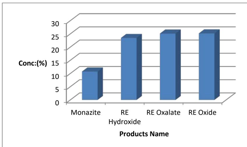
**Figure 7:** Various concentration of La<sub>2</sub>O<sub>3</sub> in rare earth oxide processing
