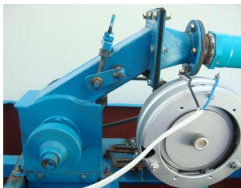
**Figure 3:** Cross-Flow Turbine
