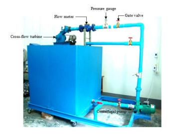
Figure 4: Experimental Set-up of Cross-flow Turbine
