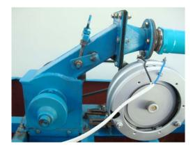
Figure 3: Cross-Flow Turbine
