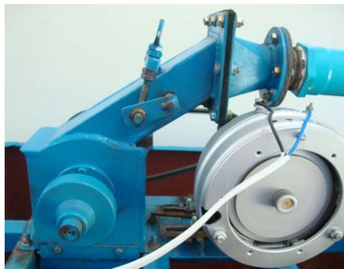
**Figure 3:** Cross-Flow Turbine
