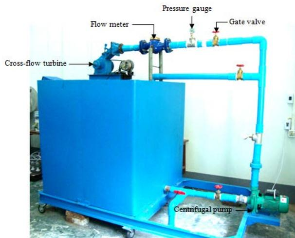
**Figure 4:** Experimental Set-up of Cross-flow Turbine
