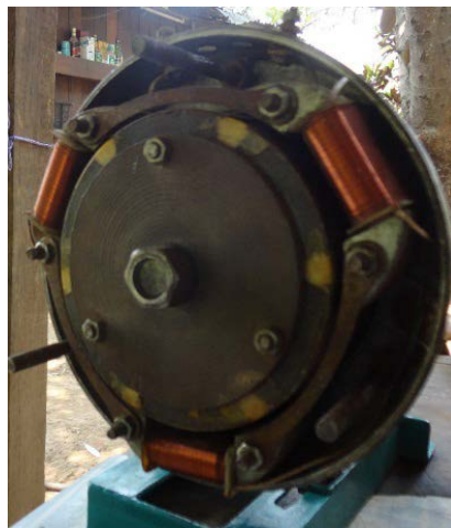
Figure 27: 300 watts generator for water turbine
