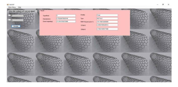
Figure 4: Simulation for metallic tube.
