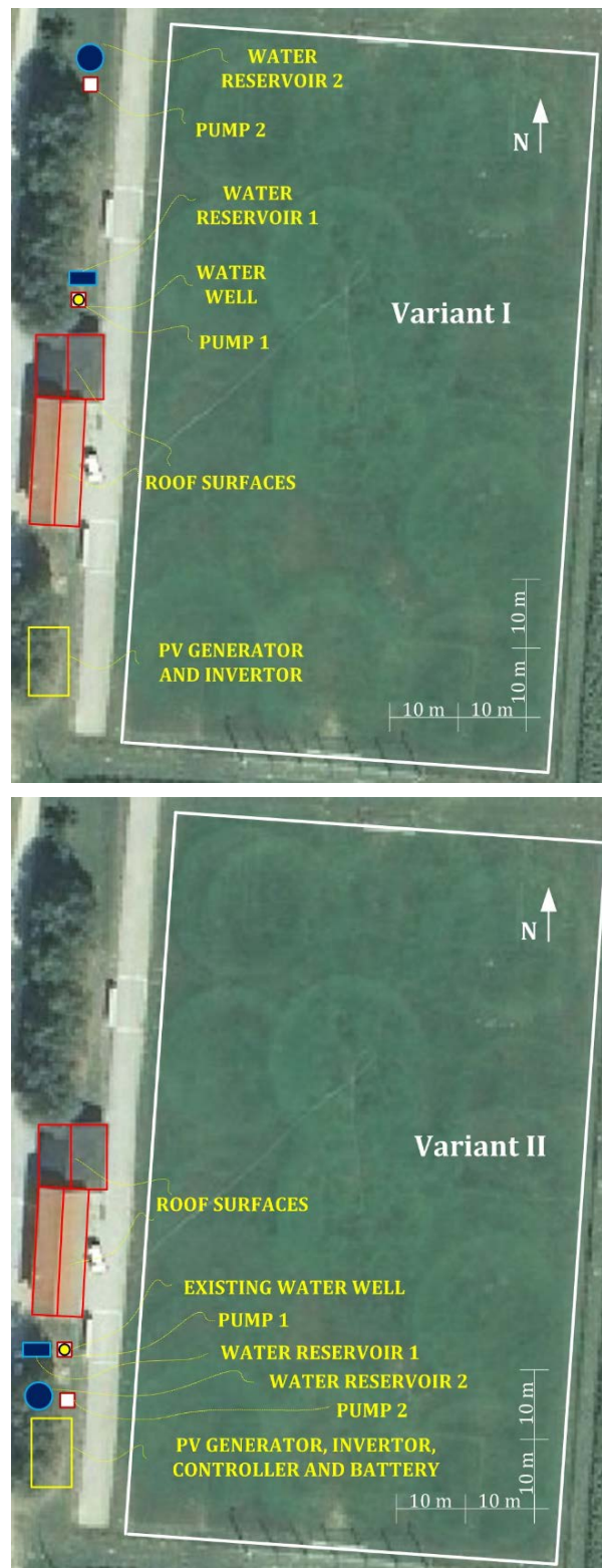
Figure 5: Schematic ground plan view of the football pitch irrigation for Variants I and II
