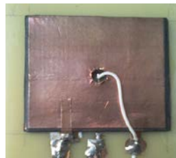
Figure 2: Photograph of integrated LC filter prototype
