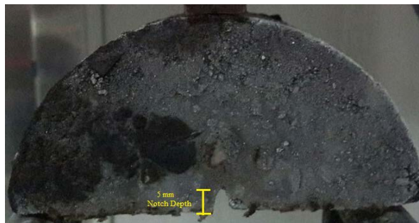
Figure 9: Semi – Circular Specimen with Notch Depth of 5mm.
