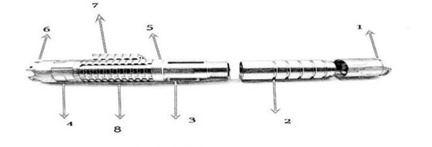
**Figure 5:** laser device, which consists of a power connector unit 1, an AC adapter 2, a laser driver 3, small dedicated actuator 4 to act as a focusable mechanism, to control the beam from the pointer 6, a cooling fan 7 to cool the laser chamber 8, and all are housed in a metal housing 5.
