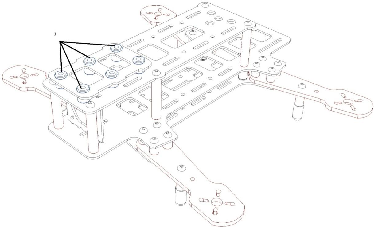
**Figure 4:** a schematic detailed drawing of the hull and the place of installing the control unit
