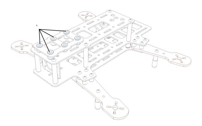
Figure 4: a schematic detailed drawing of the hull and the place of installing the control unit
