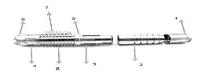
**Figure 5:** laser device, which consists of a power connector unit 1, an AC adapter 2, a laser driver 3, small dedicated actuator 4 to act as a focusable mechanism, to control the beam from the pointer 6, a cooling fan 7 to cool the laser chamber 8, and all are housed in a metal housing 5.
