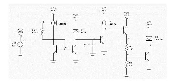
Figure 6: an exemplary circuit for the laser driver.
