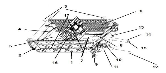
**Figure 9:** a schematic of the control unit, of a light metal housing 1 a mechanism to adjust its dimensions 2, screw cases 3, housing 4 for the laser drive, four 26650 4.2 V Li-ion rechargeable batteries 5, housing 6 for the batteries 7, detector 11, motor 9, linear actuator 10, antenna 12, laser chamber 14, pointer 15, CPU 16, an active cooling 17 mechanism using cooler fans, a receiver/transmitter 8 planted therein and connected to the CPU.
