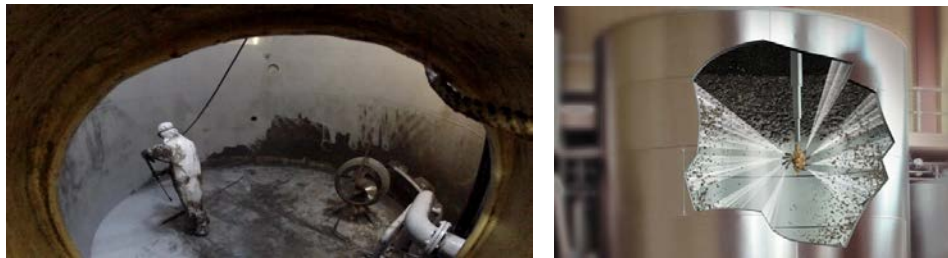
Figure 1: Water-blasting technique, a worker in confined space using a high pressure gun to clean a mud tank on an oil rig support (left), Tank cleaning by lowering a water blasting nozzle inside the tank (right)
