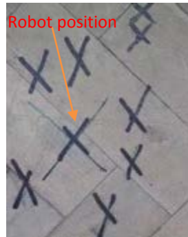
Figure 7: Errors in robot positions marked on the ground at the end of each cycle.
