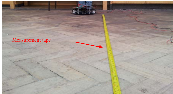
Figure 8: using a measure tape and stopwatch to measure the robot linear and velocities.
