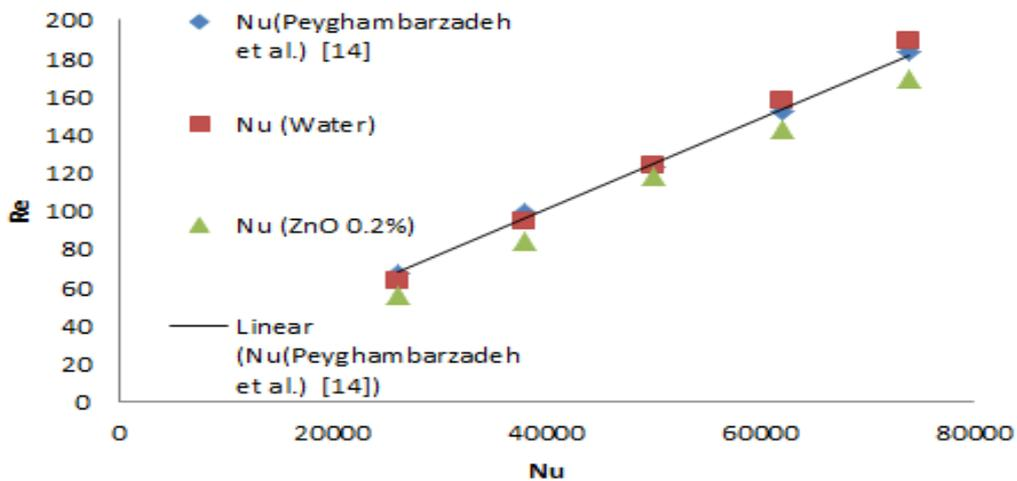
**Figure 3:** Comparison of Experimental Results of pure water and ZnO at 0.2% with the Peyghambarzadeh and his colleagues [14].
