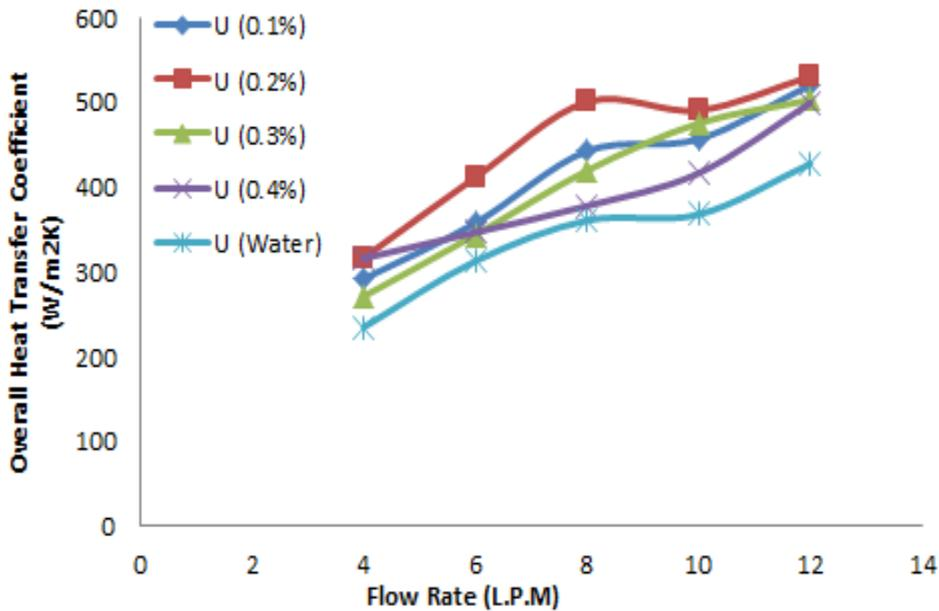
Figure 5: Overall Heat Transfer Coefficient and Flow Rate
