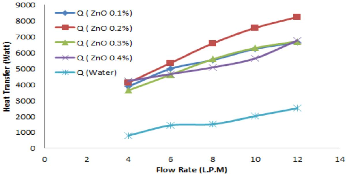
Figure 4: Heat Transfer comparison between water and different concentrations of ZnO Nanofluid
