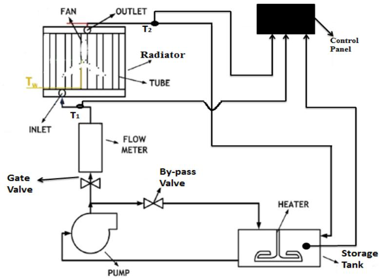
Figure 2: Line Diagram of experimental setup
