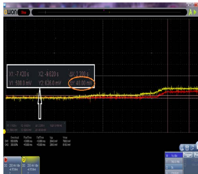
Figure 14: accuracy test of servo motor
