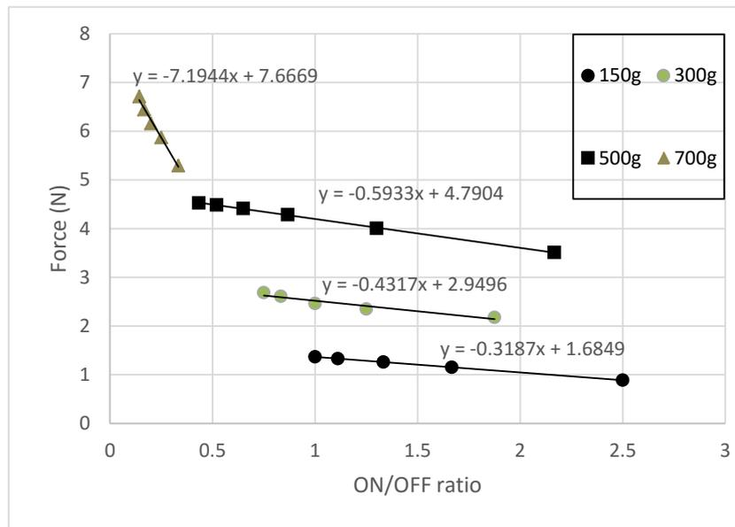
**Figure 4:** Relation between on-off ratio and represent force.
