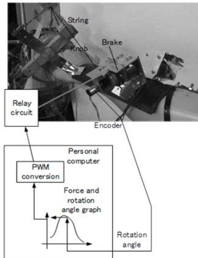
**Figure 2:** Haptic system configuration
