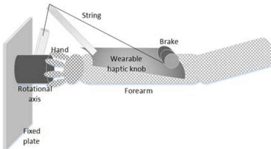
**Figure 1:** Concept of haptic knob
