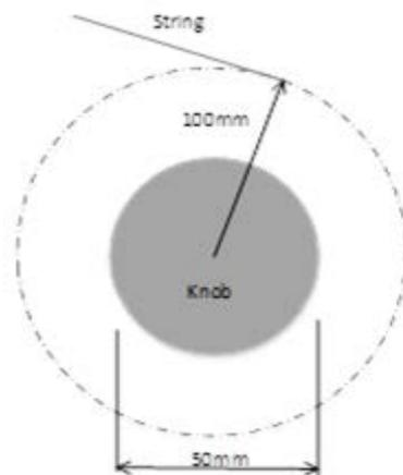
**Figure 5:** Configurational dimension of haptic display
