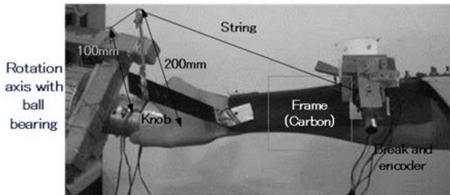
**Figure 3:** Wearable haptic mechanism.
