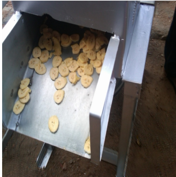
Figure 6: Sliced plantain (chips) produced by the slicing machine
