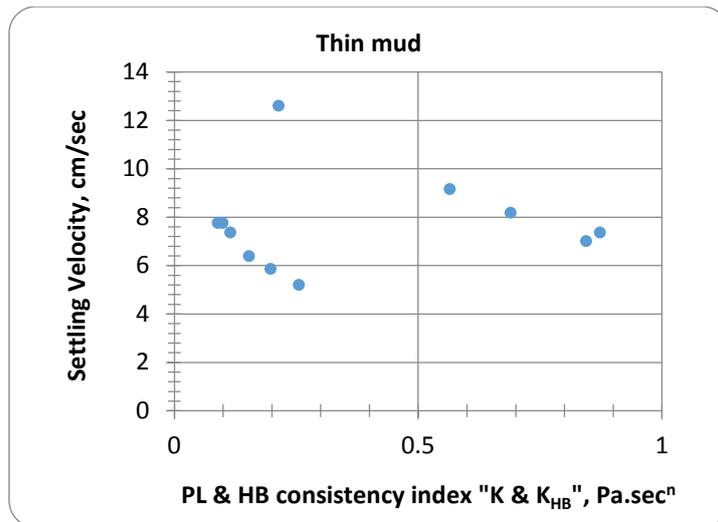
**Figure 7:** Effect of consistency index on settling velocity
