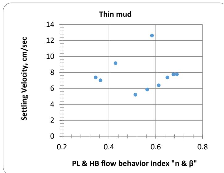
Figure 6: Effect of flow behaviour index on settling velocity
