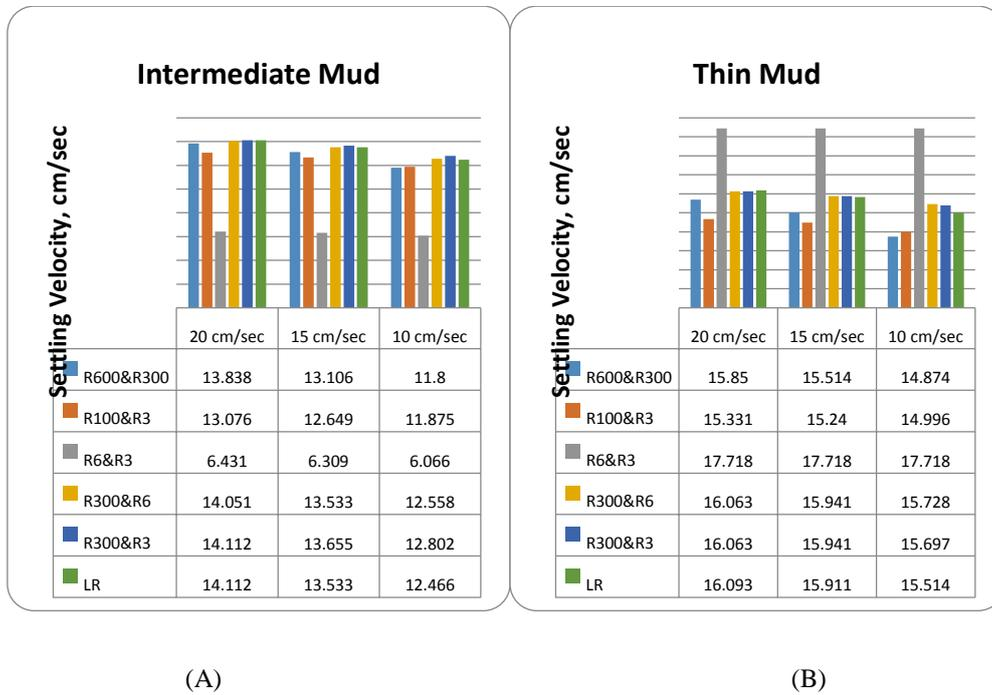
Figure 2: Chien [5] dynamic particle settling velocities – BP rheological parameters
