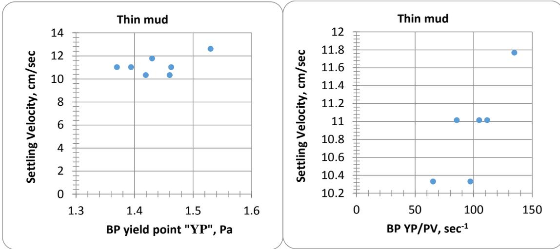
Figure 9: Effect of BP yield point and YP/PV on settling velocity
