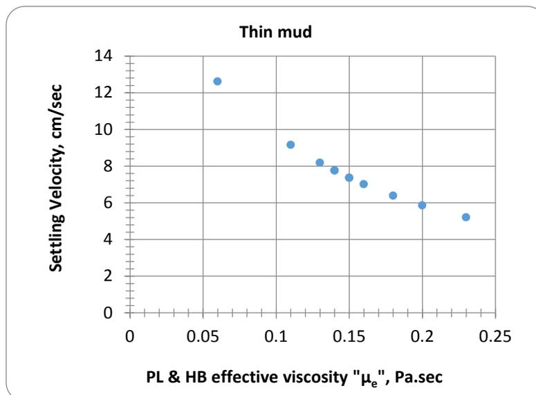
**Figure 8:** Effect of effective viscosity on settling velocity
