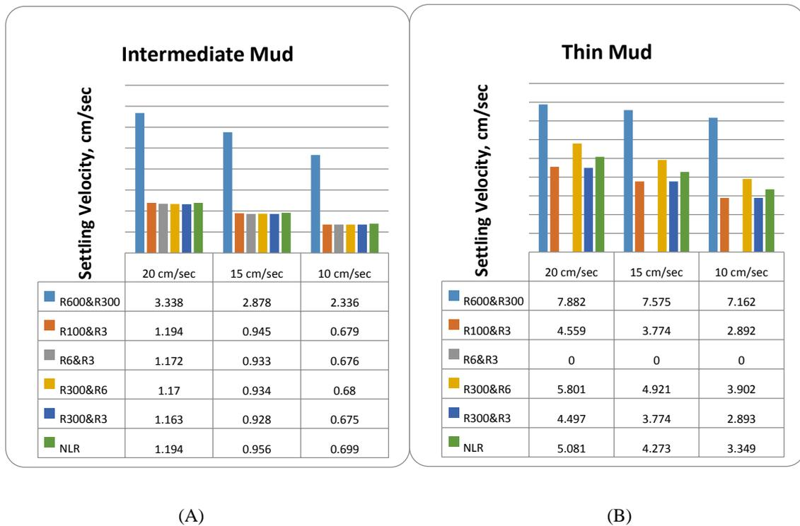
**Figure 1:** Moore [7] dynamic particle settling velocities – PL rheological parameters
