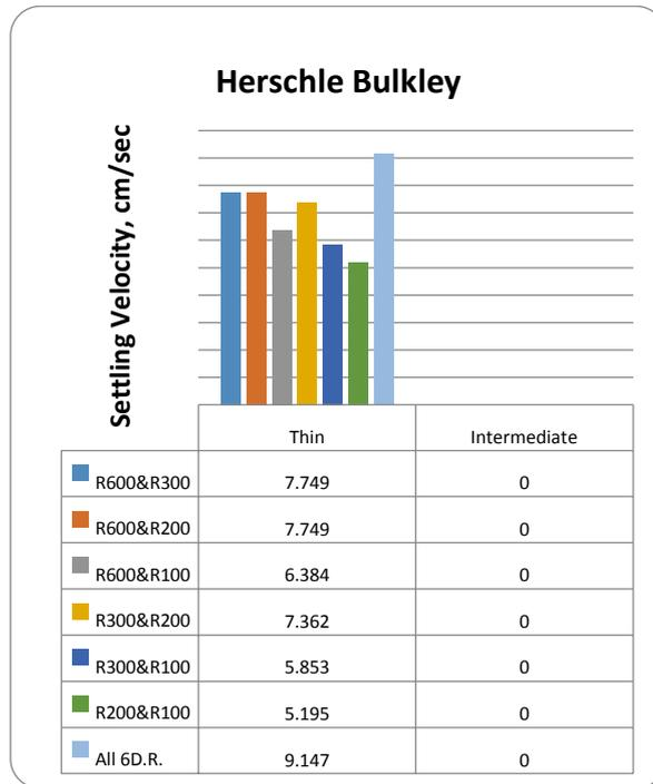
**Figure 4:** Chien [10] static particle settling velocities HB model
