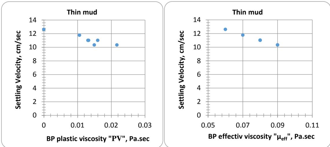
Figure 10: Effect of BP plastic and effective viscosities on settling velocity
