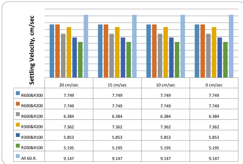
Figure 5: Chien [10] dynamic particle settling velocities in thin mud - HB model
