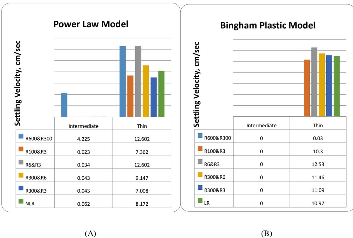
Figure 3: Chien [10] static particle settling velocities BP & PL models
