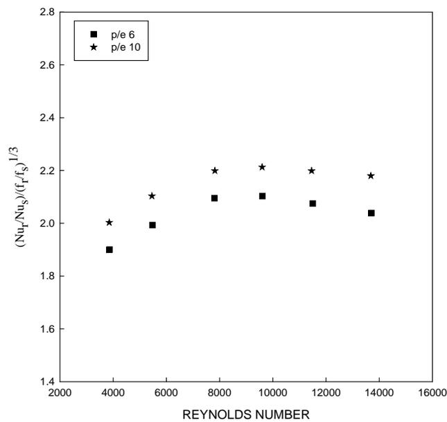
**Figure 6:** Effect of Reynolds number on Thermo-hydraulic parameter for relative roughness pitch as compare to smooth duct for W-discrete ribs flow arrangement.
