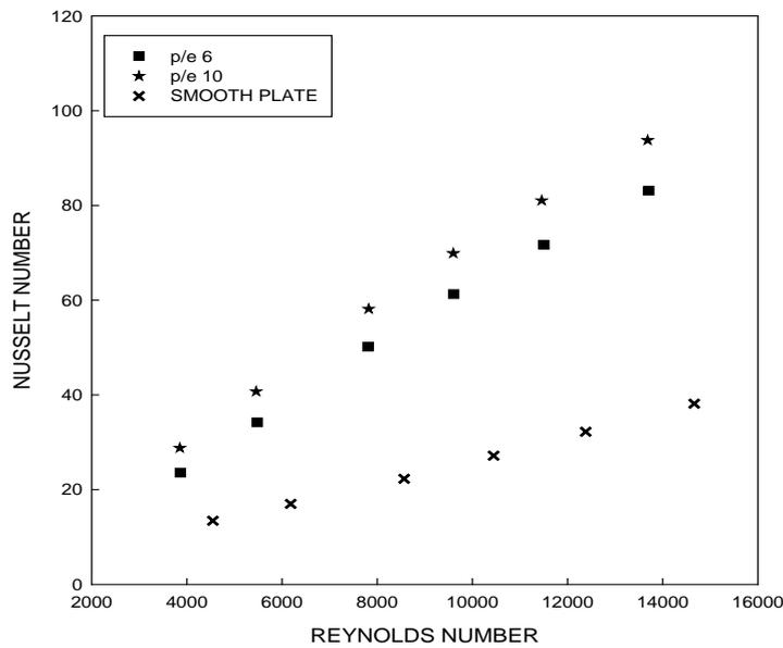
**Figure 4:** Effect of Reynolds on Nusselt number with variation of relative roughness pitch as compare to smooth duct for W-discrete ribs flow arrangement.
