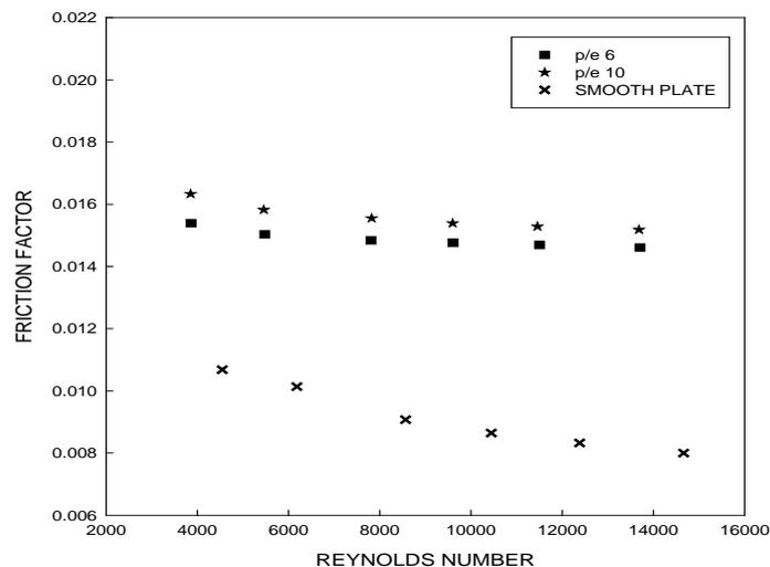
**Figure 5:** Effect of Reynolds on friction factor with variation relative roughness pitch as compare to smooth duct for W-discrete ribs flow arrangement.
