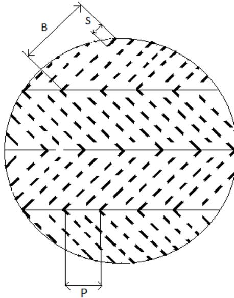
**Figure 3:** Enlarged view of cross-section of roughness plate
