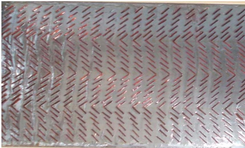
Figure 2: Photograph of W-discrete ribs roughness plate
