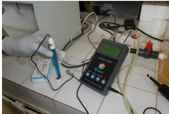
Figure 5: PH meters digesters
