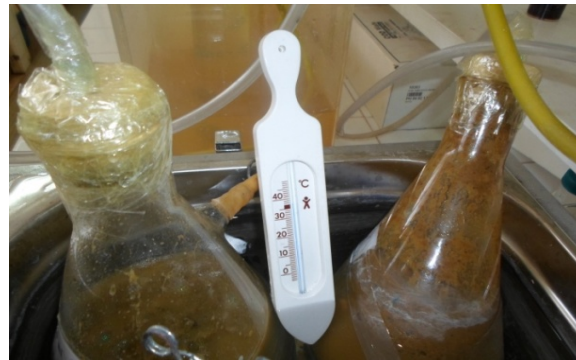
Figure 3: Measuring temperature digesters
