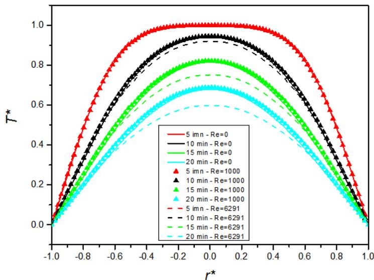
**Figure 10:** Comparison of the dimensionless radial temperature distribution at constant wall temperature with 5 minutes interval time for 3 different Reynolds numbers ( $Re = 0$ ;  $Re = 1000$ ;  $Re = 6291$ )
