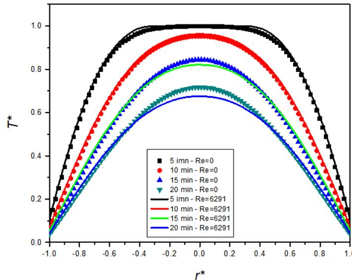
**Figure 8:** Dimensionless radial temperature distribution at constant heat transfer coefficient with 5 minutes interval time for two different Reynolds numbers (Re = 0; Re = 6291)
