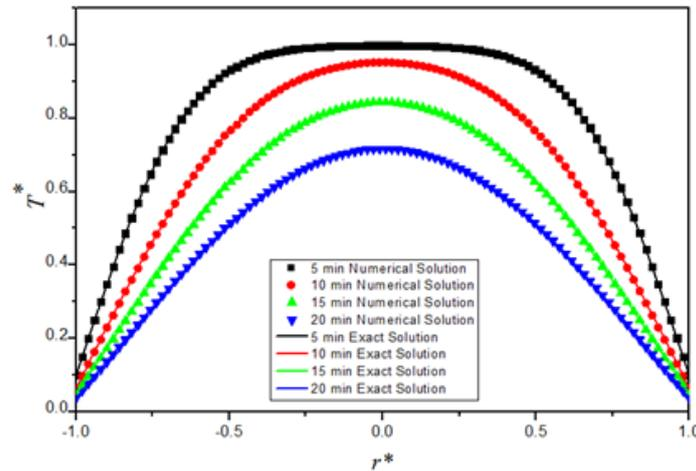
**Figure 4:** Comparison between the numerical and analytical temperature distributions at different time steps
