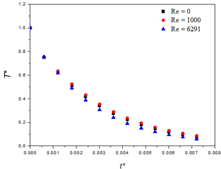
**Figure 11:** Average temperature distribution for different Reynolds numbers
