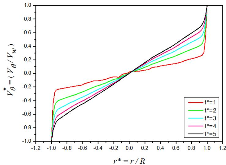
**Figure 6:** Dimensionless velocity distribution at different  $t^*$
