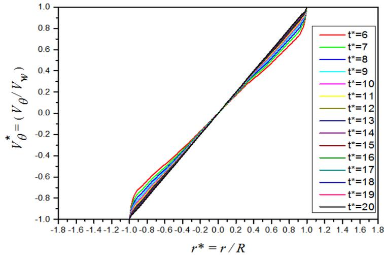
**Figure 7:** Dimensionless velocity distribution at different  $t^*$
