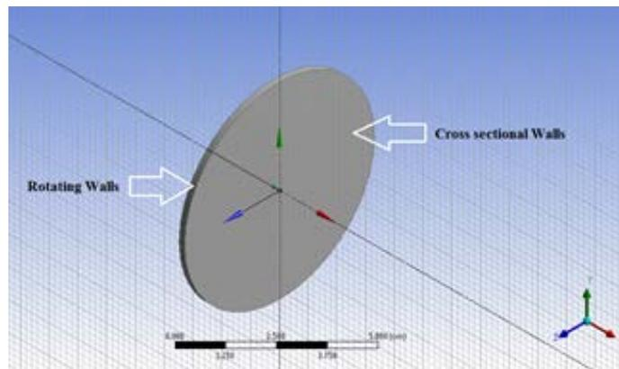
**Figure 2:** 3D geometry of the full disk as simulated in ANSYS FLUENT
