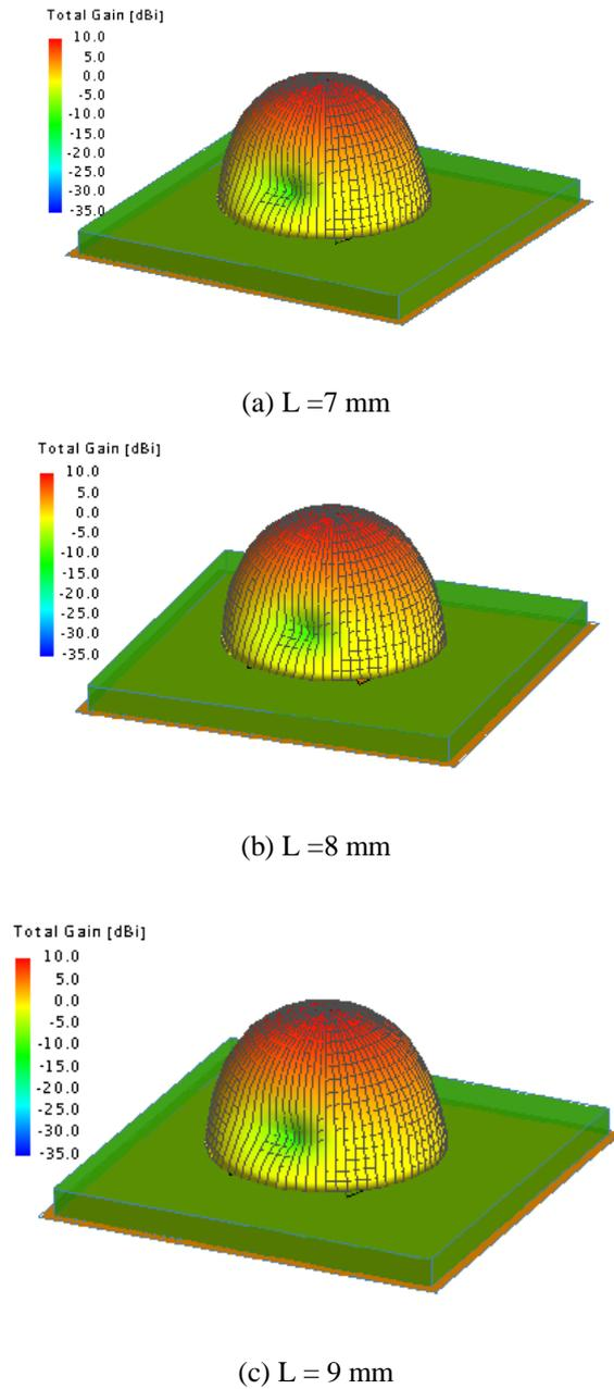
**Figure 5:** 3-D dimension results of gain produced by FEKO in x-y plane at resonant frequency (a):  $f = 12.57$  GHz (b):  $f = 12.61$  GHz (c):  $f = 12.62$  GHz
