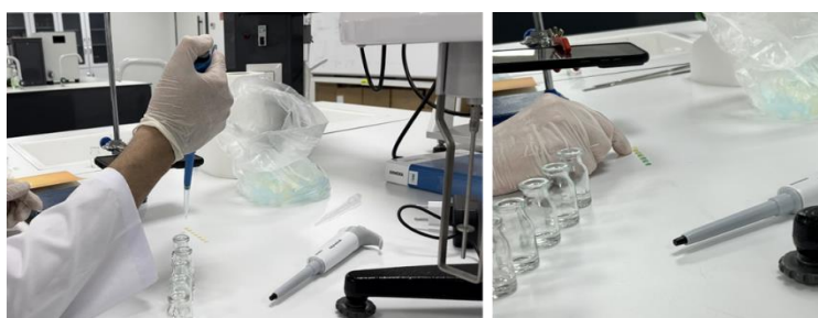
Figure 2: For this purpose, lyophilized BSA was dissolved in ultrapure water at a concentration range of 0.075 - 0.15 g/L at room temperature and interacted with the sensor surfaces
