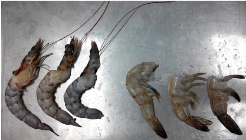
Figure 2: Separation of shrimps' meat from their shells after a 345 MPa treatment
