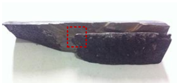
Figure 10: Observation area of microstructure and SEM image marked with a red dotted line
