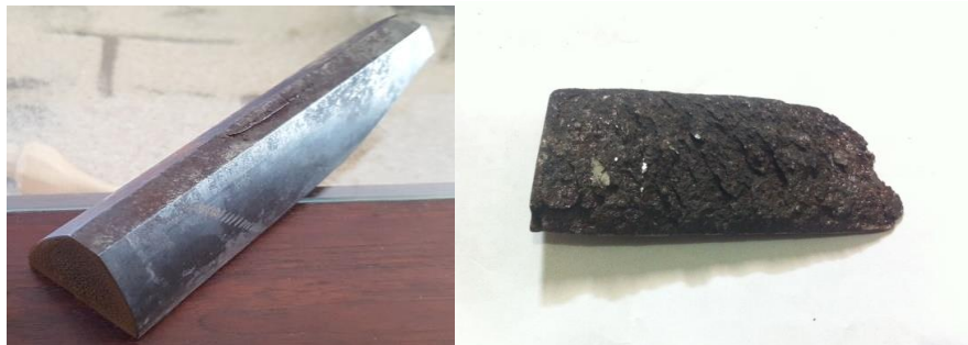
Figure 5: Fault spur gear (left) and Fracture surface of fault spur gear (right)
