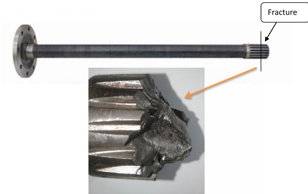
Figure 1. The broken of the axle shaft whos connected with a differential gear
