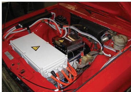
Figure 13: EV Conversion of Opel Kadett C 1978, University of Zagreb, Dubrovnik, Croatia - 2014 [25]
