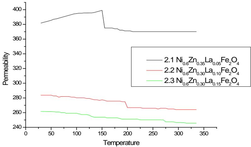
**Figure 3:** Temperature dependence of the real part of the permeability, as a function of Temperature of  $Ni_{0.60}Zn_{0.35}La_{0.05}Fe_2O_4$ ,  $Ni_{0.60}Zn_{0.30}La_{0.10}Fe_2O_4$  and  $Ni_{0.60}Zn_{0.25}La_{0.15}Fe_2O_4$  sintered at  $1250^{\circ}C$
