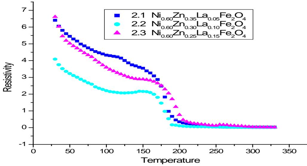
**Figure 1:** Temperature dependence of resistivity, as a function of Temperature of  $\text{Ni}_{0.60}\text{Zn}_{0.35}\text{La}_{0.05}\text{Fe}_2\text{O}_4$ ,  $\text{Ni}_{0.60}\text{Zn}_{0.30}\text{La}_{0.10}\text{Fe}_2\text{O}_4$ , and  $\text{Ni}_{0.60}\text{Zn}_{0.25}\text{La}_{0.15}\text{Fe}_2\text{O}_4$ , sintered at  $1250^\circ\text{C}$
