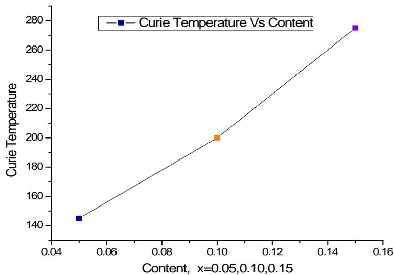
**Figure 4:** Curie temperature dependence of the content, as a function of Temperature of  $\text{Ni}_{0.60}\text{Zn}_{0.35}\text{La}_{0.05}\text{Fe}_2\text{O}_4$ ,  $\text{Ni}_{0.60}\text{Zn}_{0.30}\text{La}_{0.10}\text{Fe}_2\text{O}_4$  and  $\text{Ni}_{0.60}\text{Zn}_{0.25}\text{La}_{0.15}\text{Fe}_2\text{O}_4$  sintered at  $1250^\circ\text{C}$
