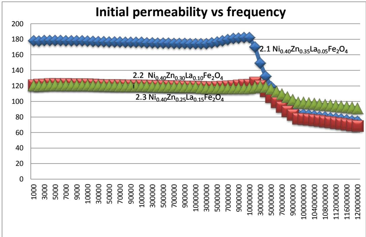
**Figure-2:** Frequency dependence of the real part of the permeability, as a function of frequency of  $\text{Ni}_{0.60}\text{Zn}_{0.35}\text{La}_{0.05}\text{Fe}_2\text{O}_4$ ,  $\text{Ni}_{0.60}\text{Zn}_{0.30}\text{La}_{0.10}\text{Fe}_2\text{O}_4$  and  $\text{Ni}_{0.60}\text{Zn}_{0.25}\text{La}_{0.15}\text{Fe}_2\text{O}_4$  sintered at  $1250^\circ\text{C}$
