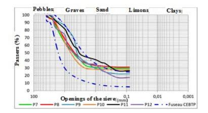
Figure 5: Particle size curves of Bakoye samples poorly inscribed in the standard spindle recommended by the [13] as a base layer.
