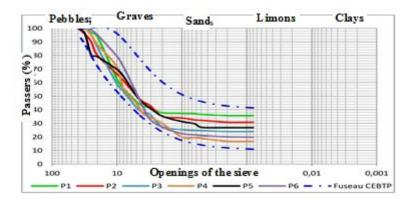
Figure 2: Granulometric curves of Banfeko samples relatively well inscribed in the standard recommended by [13] as a subbase
