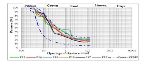
**Figure 7:** Particle size curves of Ketcho samples poorly inscribed in the standard spindle recommended by the [13] as a base layer.
