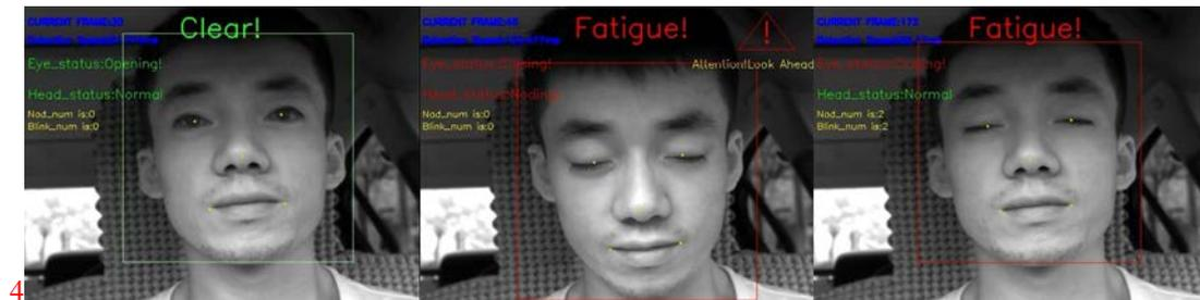
**Figure 6:** The screenshots of real-time fatigue driving detection on embedded platform
