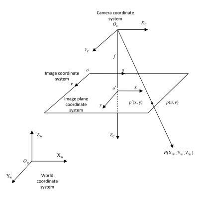
Figure 4: Perspective projection model
