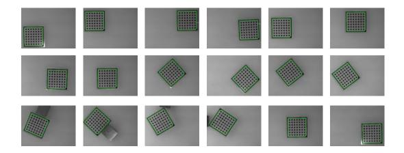
Figure 6: Calibration board images under different postures
