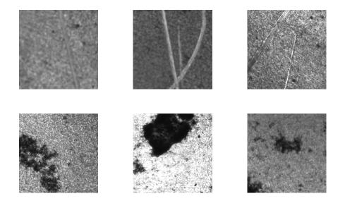
Figure 7: Scratches and rust
