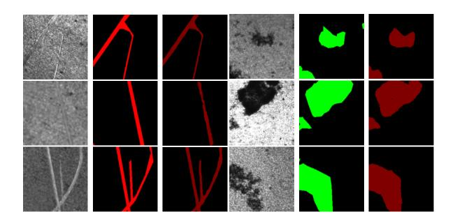
Figure 9: The segmentation results of scratches and rust
