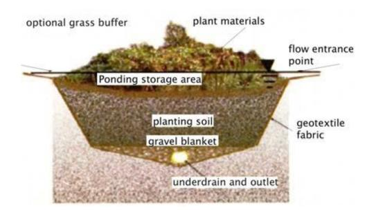
Figure 3: Typical Illustration for Bioretention Area
