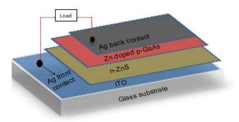
Figure 1: Structure of solar cell on glass substrate with double action p-n junction.
