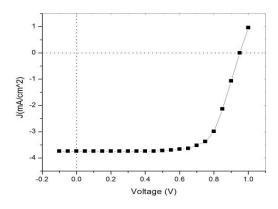
Figure 7: J-V charecteristic curve under illumination.
