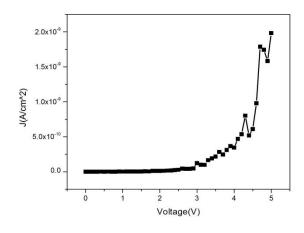
Figure 4: Dark I-V characteristics of cell
