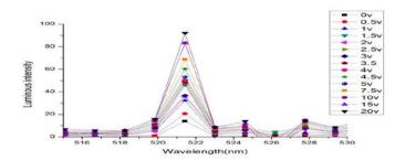
Figure 8: Luminescence Spectra of device in reverse bias.
