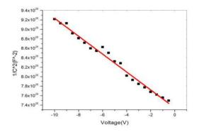
**Figure 6:**  $1/C^2$  VS reverse V (voltage) at 100 KHz.
