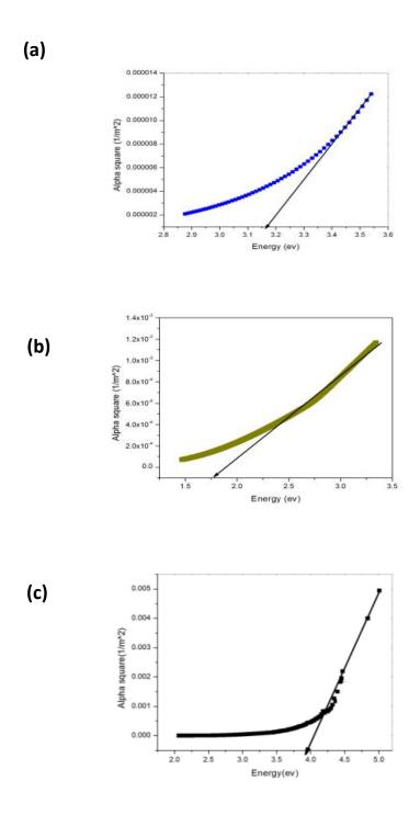
Figure 3: Optical Band gap of thin film of (a) ITO (b) Zn doped GaAs(1:2) (c) ZnS
