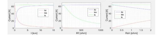
Figure 5: Dependences of the fault currents model without load - isolated network
