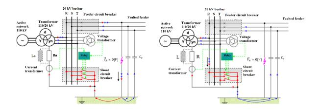
Figure 1: Operation principle of shunt circuit breaker left (off), right (on)
