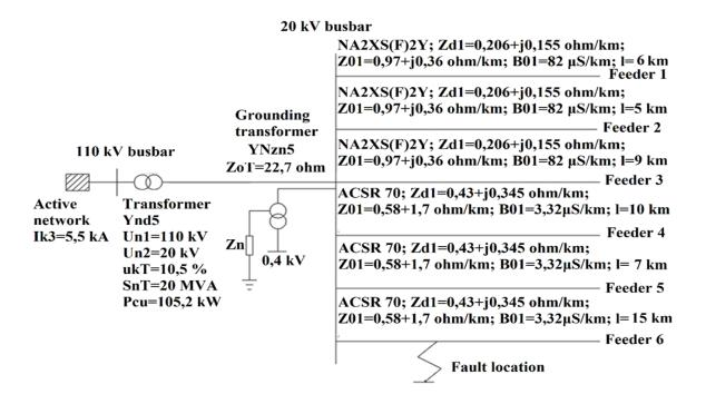
Figure 4: Case study 20 kV distribution network
