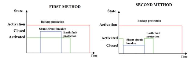
Figure 2: Coordination between the shunt circuit breaker operation and definite-time earth fault protection
