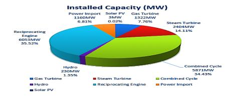
Figure 12: Technology wise power generation capacity (MW) of Bangladesh in year 2018 [10]
