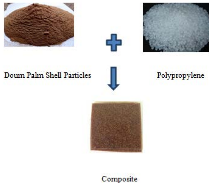
Figure 3: Doum palm shell particles and polypropylene Composite
