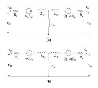
Figure 1: (a) d-equivalent circuit of IM (b) q-equivalent circuit of IM.
