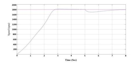
Figure 4: Rotor Speed in Closed Loop with 200 N.m load (r.p.m).
