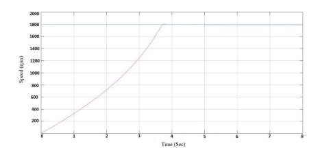
Figure 8: Rotor Speed with FLC (r.p.m)
