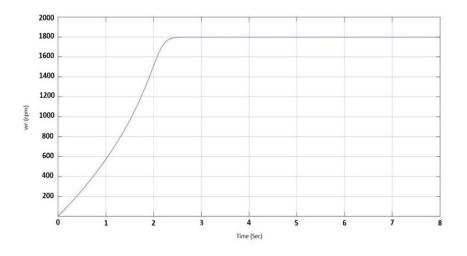
Figure 2: Rotor Speed, open loop system with No Load (r.p.m).
