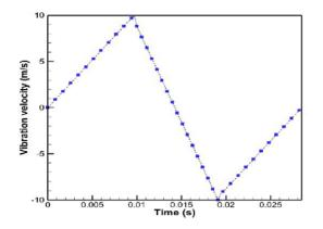
Figure 2: Evolution of hot air velocity during a period for triangular vibration
