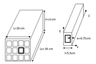
Figure 1: Whole clay brick dimensions.
