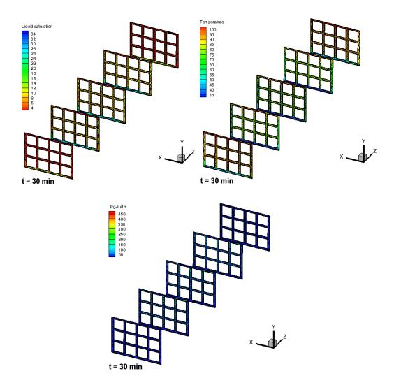
Figure 10: Distribution of the temperature, the liquid saturation and the gaseous pressure after 30 minutes.
