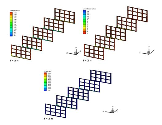
Figure 12: Distribution of the temperature, the liquid saturation and the gaseous pressure after 2h.
