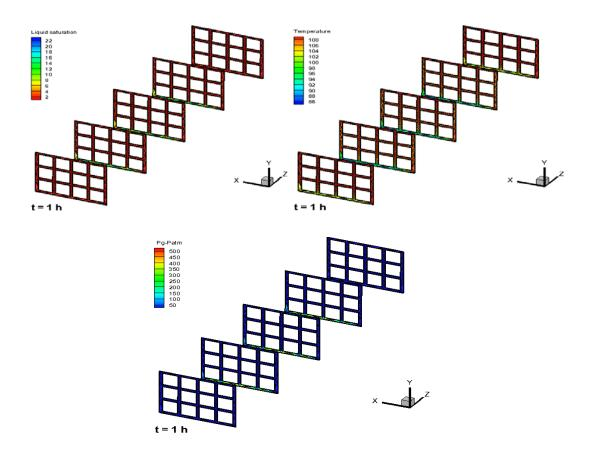
Figure 11: Distribution of the temperature, the liquid saturation and the gaseous pressure after 1h
