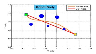
Figure 3: Difference between two paths of obstacles avoidance without and with applying PSO case 2
