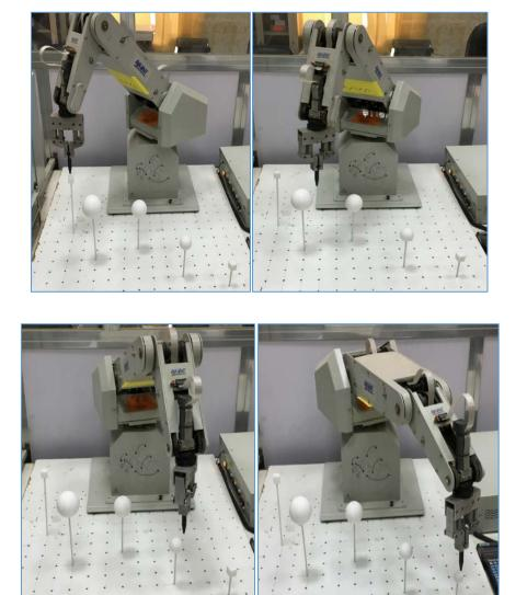
Figure 5: Physical steps case 1 of three obstacle avoidance path planning in the real environment
