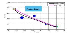
Figure 4: Two path planning of obstacles avoidance without and with applying PSO case 1
