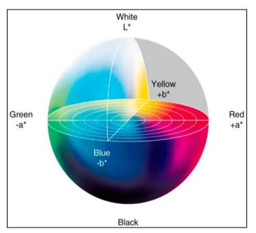
Figure 1: L\*a\*b\* color space measurement [adapted from https://largeinkjet.wordpress.com/tag/lch/]
