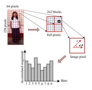
Figure 4: Histogram of Oriented Gradients Overview
