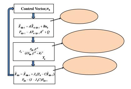
Figure 12: Flowchart of the Kalman filter used for human tracking system
