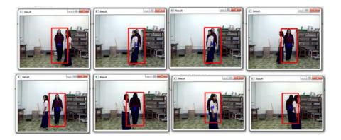
Figure 14: Processing results for target human tracking in occluded condition using Kalman filter
