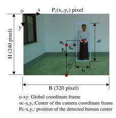
Figure 10: Position of a human in the camera coordinate frame fixed to a camera
